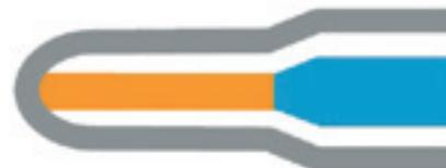
The swaging can be used on heating elements without cold ends as well with cold ends.
